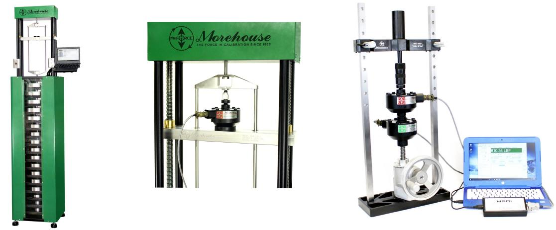
Tier 1: Primary Standard 0.0016 % used to calibrate Secondary Standards to Class AA
