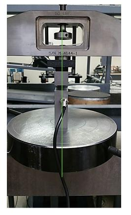
Output in mV/V Aligned in machine -1.96732 mV/V
