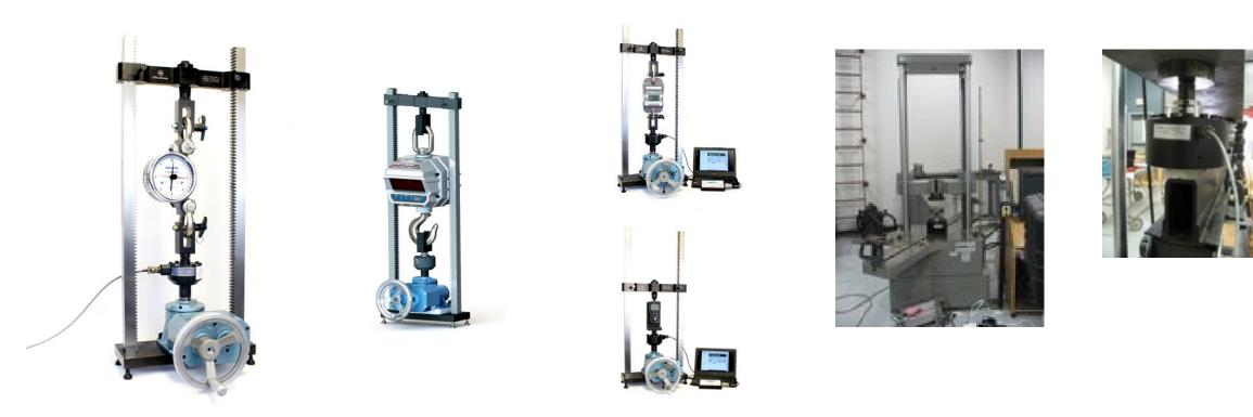
Tier 3 :Calibration of Working Standards using a Comparator (Morehouse Bench Top machine with load cell) to calibrate various different equipment. CMC's typically vary from 0.03 % to 0.5 %.
